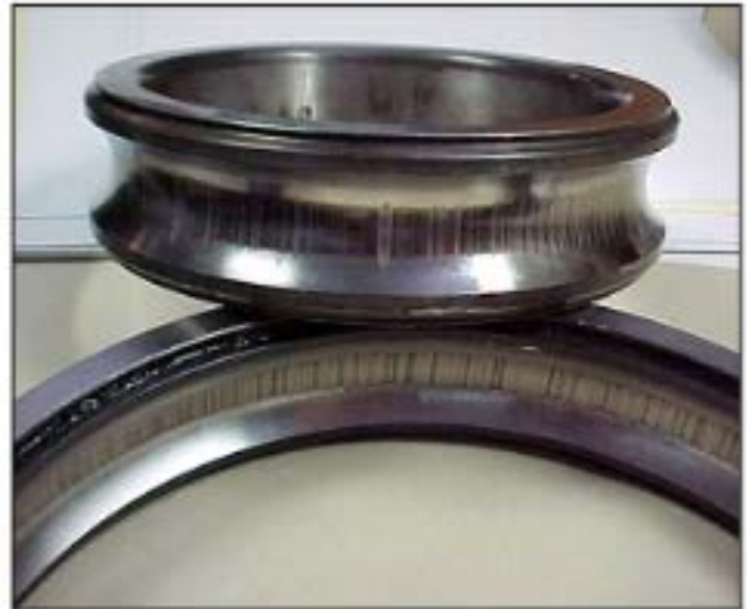
Fluting of the bearing races due to electrical current.
