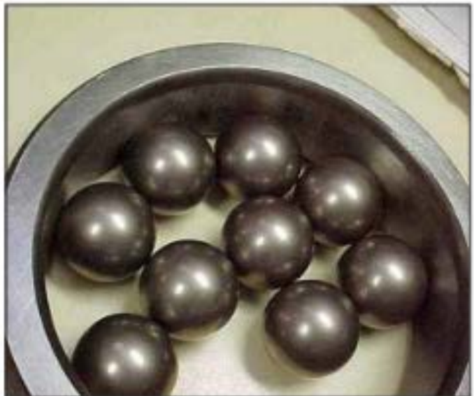
Frosting of the balls/rollers due to electrical current.
